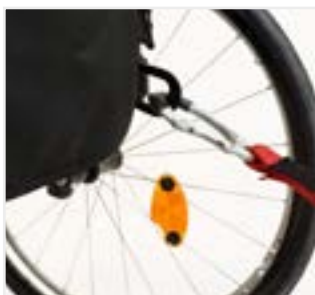
// QSS090100 Tie down brackets for transportation according to ISO 7176-19 (max. user-weight 136 kg)
